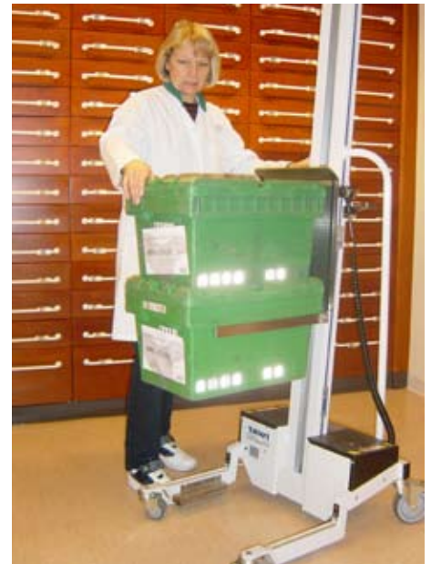
Crates in stacks are handled with a fork tool on PRO70.
